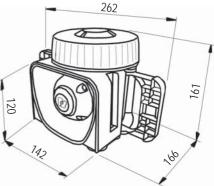
LM500-D Solaris Series dimensions (mm).
